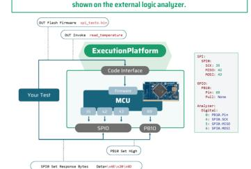
Example Endpoint configuration for SPI and a single GPIO. All pins are
